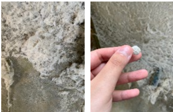
Figure 8: The Rest of The 'Cotton' Processing of Pineapple Fibers on the Decorticator Machine Source: Author,2021
