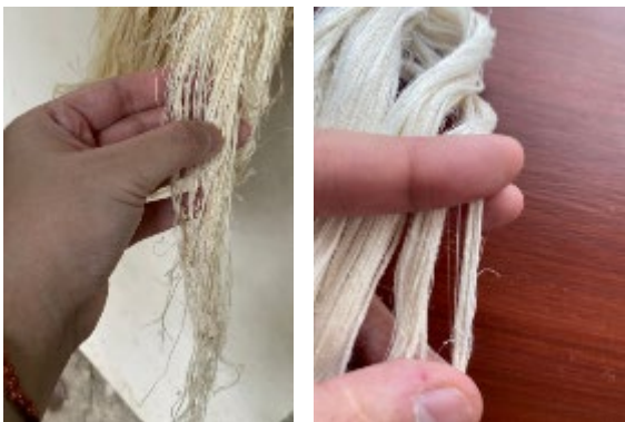
Figure 9: Comparison of Fibers Before and After Mashing Source: Author, 2021
