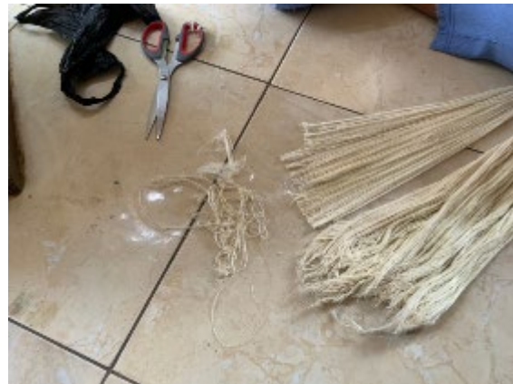
Figure 10: Combed and Uncombed Fibers and The Residue of the Combing Process. Source: Author, 2021
